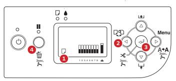
Plug USB cable from the printer into the computer you are using. Make sure sheet icon is showing at bottom of display (1). If it is not, press the sheet/roll selector button (2) until it is.
